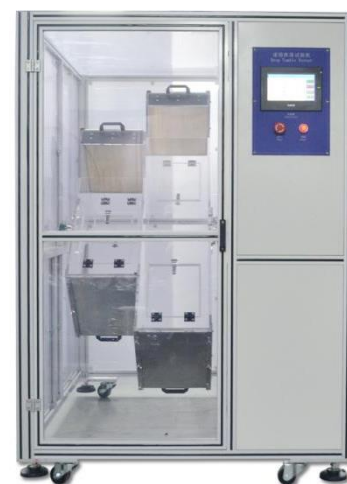
Model : SR-220A Tumble drop tester Protect cover + 0.5m + 1m
