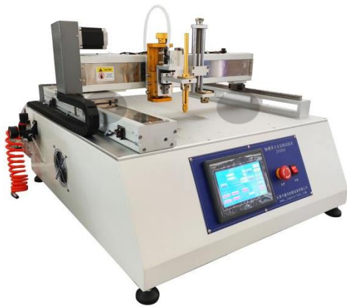
SR-207 Click and Line Life tester Can test click and line testing for Touch screen
