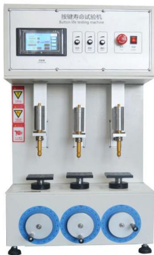
SR-211 Button life tester Suitable for small buttons, can add weights
